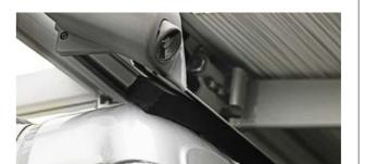
308697 - Black EPDM foam strip with closed cell structure to seal the gap between the vehicle and a roof-mounted awning.
